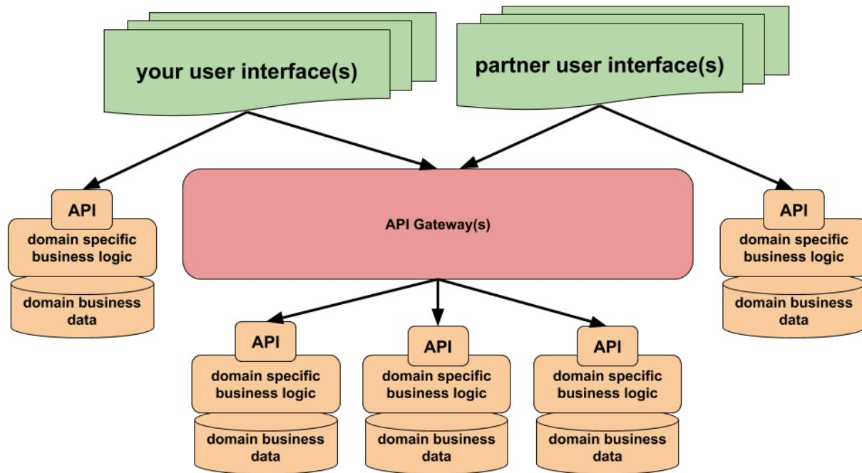
In Service Oriented Architecture cloud-nativeness is more widely adapted. User interfaces are decoupled from backend logic over APIs and can be scaled independently. API gateway scale is still a problem and the majority of services are likely to be virtual machine stacks that are running and supporting their API functionality. This is a slightly easier problem to scale, but peak hours can still impact increased costs and requirements.
