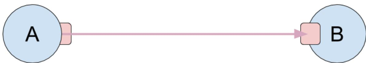
Service A wishes to request data from service B over X-Road. This request is a synchronous request, meaning that service A will be waiting for a response from service B.
