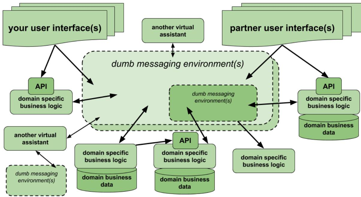
In microservice architecture every component can be scaled individually if deployed to cloud, such as AWS. While this is a very simplified model, if all services and service components are in cloud, then they can be scaled per single component demand. If good principles for microservice architecture are kept in mind, then cloud platform is able to scale components in a dynamic manner<sup>81</sup> by creating multiple instances temporarily to deal with the load.
